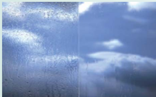
Figure B24.2 Windows with and without a photocatalytic self-cleaning layer.
